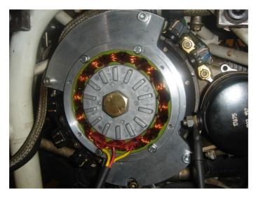
We are pleased to present the FLYGAS ALTERNATOR KIT, the ideal solution for boosting the electricity on board the ROTAX engine of the ULM (ultra light airplane.) adding a spare alternator unit.
